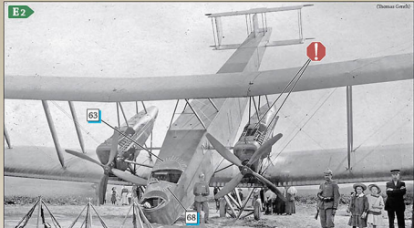
Handley-Page O/100 3134 "A 1" resting gently on its nose after landing behind German lines. Note the 34 gradient points of the compass painted around the cockpit [63] & [68] and that various engine nacelle panels have been removed to improve cooling.
