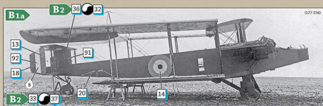
Handley-Page O/100 1463 "L'Amazone" with its wings folded and propellers and nacelle rear fairings removed. Various components have been marked "R.A." etc by the Germans to simplify reassembly. The mottled appearance of the underside of the top wing appears to be an optical illusion caused by the roughly hand painted finish exhibiting a mix of semi-gloss and matt that are reflecting the bright snow covered background differently.
