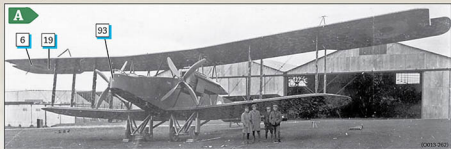
^ v Two views of Handley-Page O/100 1459 at No.3 Wing in Ochey during March 1917. Note the mottled camouflage finish on the interplane struts, undersides of the wings and fuselage (and presumably tailplane) which appears to be PC10 over bleached linen. The engine nacelles appear to be finished in grey while the "white" areas of the wing cockades & rudder stripes appear to remain unpainted translucent bleached linen.
