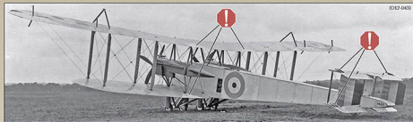
^ v Handley-Page O/100 1457 was the 3rd prototype and is seen here in the middle of 1916 in overall clear doped Irish linen with grey painted engine nacelles etc. The linen has been removed from the elevator balances to improve handling but their ribs remain in position. Note how bright the undoped linen wing fold gussets appear and that no white paint appears to have been used in the cockades or rudder stripes.
