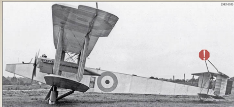
^ v Handley-Page O/100 1457 was the 3rd prototype and is seen here in the middle of 1916 in overall clear doped Irish linen with grey painted engine nacelles etc. The linen has been removed from the elevator balances to improve handling but their ribs remain in position. Note how bright the undoped linen wing fold gussets appear and that no white paint appears to have been used in the cockades or rudder stripes.
